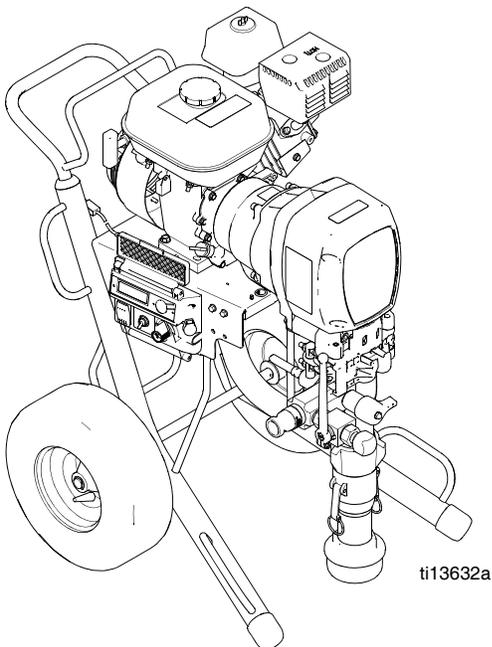
The HTX 2030 Sprayer comes equipped with a Base Coat Pump 24B321. Only water-based materials are to be used with this configuration, such as:
