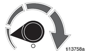
4. OFF (fully counterclockwise) - stops pump completely:
