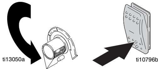
3. Unlock trigger safety. Hold metal part of gun firmly to side of grounded metal pail and trigger gun to relieve pressure.
