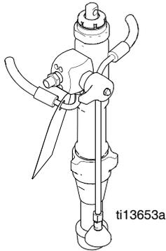
The pump on the HTX 2030 Sprayer can also be switched out with a Top Coat Kit 24B140 (**purchased separately**). This pump is used for less viscous materials such as:
