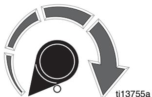
5. Adjust engine speed to control flow rate of sprayer. Start with the slowest speed possible for maximum spray control. Different spray tip nozzle sizes can also be tried.
