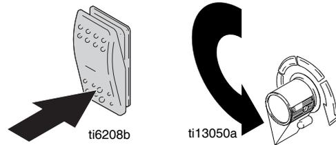
2. Turn on/off switch OFF and turn pressure control knob fully counterclockwise.
