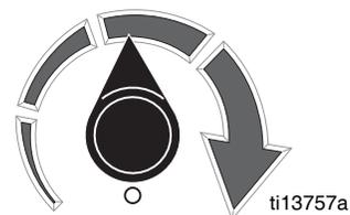
3. Flow 1 (near counterclockwise end of pump control) reduces flow more by interrupting pump longer:
