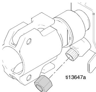
4. Turn air valve OFF. Connect applicator to material hose and air hose. Air supply minimum requirements vary with material thickness and desired thickness.
