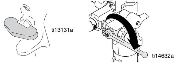
**NOTE:** If you suspect that the spray tip nozzle or hose is completely clogged, or that pressure has not been fully relieved after following the previous steps, **VERY SLOWLY** loosen the tip guard retaining nut or hose end coupling to relieve pressure gradually, then loosen completely. Then clear tip or hose.
