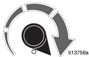
2. Flow 2 (near middle of the rotation) reduces flow slightly by briefly interrupting pump:
