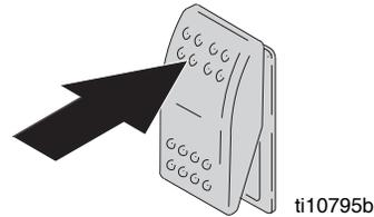
5. Hold applicator over material pail, trigger on, and turn pump ON using applicator switch on hose. **NOTE:** Remove spray disk then set material flow to prevent material from back-flowing into air passages of gun.
