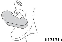
2. Turn on/off switch to OFF and turn pressure control knob fully counterclockwise.
