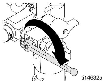
**NOTE:** If you suspect spray tip nozzle or hose is completely clogged or that pressure has not been fully relieved after following the previous steps, cover the connection at end of hose with a heavy rag and **very slowly** loosen connection.
