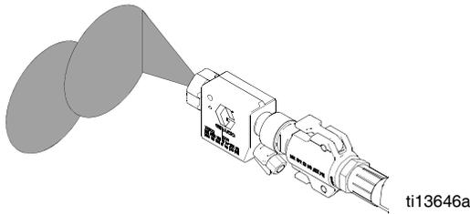
9. Adjust air valve and/or select alternative nozzle size (4 - 10mm) for desired finish.
