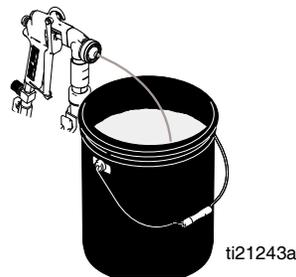
6. Turn pump control clockwise and adjust engine throttle to lowest setting until desired material delivery rate is achieved.
