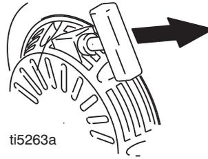
6. After engine starts, move choke to OPEN.
