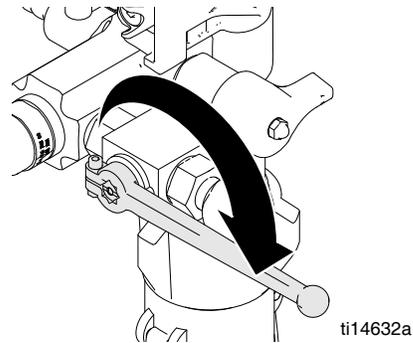
16. Turn on/off switch OFF when valve is thoroughly flushed.
