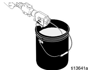
7. Turn pump control clockwise until desired material delivery rate is achieved.
