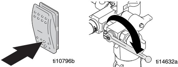
11. Connect applicator to material hose. Close prime/drain valve.
