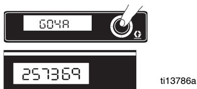
6. Short press DTS button and Base Coat hours displays.
