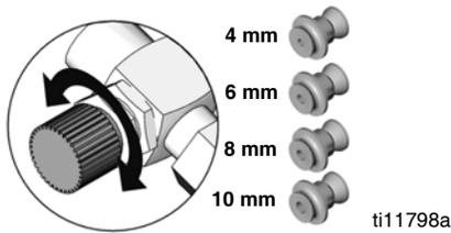
3. Turn air valve OFF. Connect applicator to material hose and air hose. Air supply minimum requirements vary with material thickness and desired thickness.
