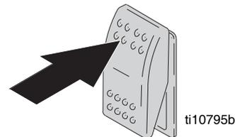
6. Hold applicator over material pail and turn pump ON using applicator switch on hose.
