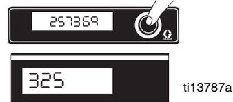
7. Short press DTS button and LAST ERROR scrolls through display followed by stored error message and error code. This information cycles repeatedly until cleared.
