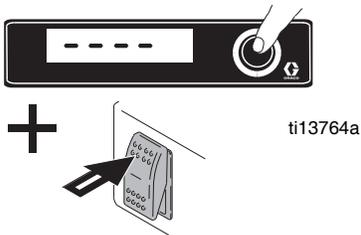
3. SERIAL NUM scrolls through display and a 3 to 5-digit serial number displays.
