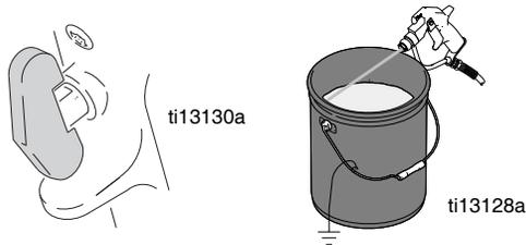
4. Lock gun trigger safety. Open pressure prime/drain valve. Leave valve open until ready to spray again.
