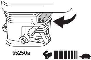
4. Set engine switch to ON.
