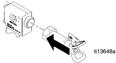
2. Insert metal seat and OneSeal. Insert Switch Tip. Screw assembly onto applicator.
