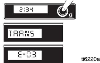
8. Press and hold DTS button until CLEAR ERROR NO ERROR CODE scrolls through the display and error code E=00 displays.
